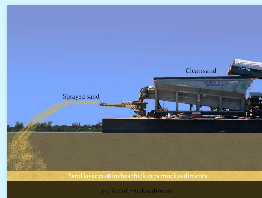
Figure 7: Sand shooter diagram.
